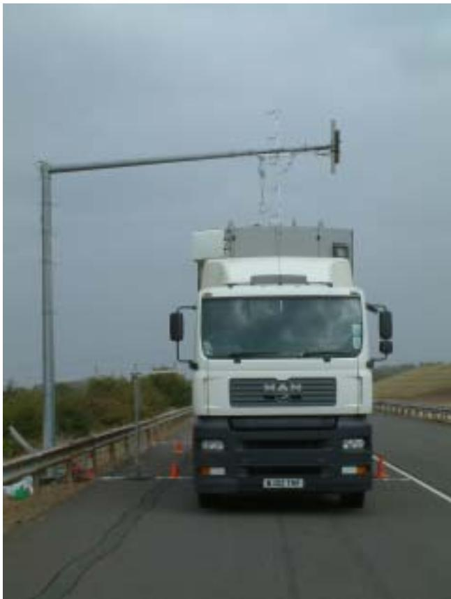
some 4 m high and 15 m long. The vehicle will be driven at different speeds and at different positions beneath the structure. The pressure wave, wake flow, and structural response will be monitored to provide the understanding and data needed to formulate fatigue design rules.
